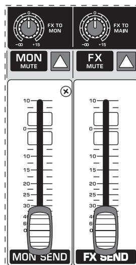
Fig. 2.6: Aux send controls of the main section
