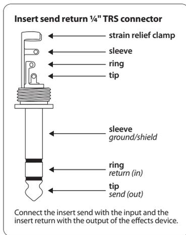
Fig. 4.5: Insert send return 1/4" TRS connector
