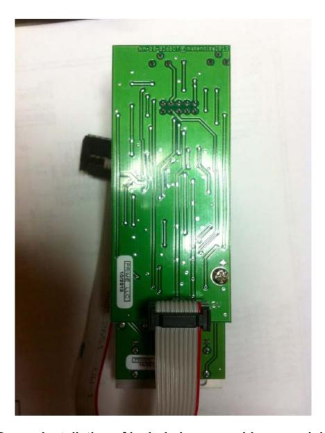
Proper installation of included power cable on module. Please note the RED BAND.
