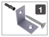
Using suitable screws and wall plugs, fix 2 L Brackets to the wall at the correct height to support the bottom edge of your tile. They should be located approximately 20mm in from the corners of the tile.
