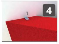
Push your tile between the brackets. Fix 4 suitable screws into the MDF edging of the tile. We recommend using a 'pan head' wood screw.
