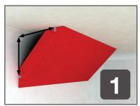
Fix one bracket to the ceiling and one to the wall. If using a corner trap, each should be 315mm from the corner. Note that the corner may be hidden behind the coving! If so just offer the trap up and mark it.
