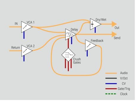
signal at slow rates in different ways, depending of the position of the three **Crush** switches or by the presence of gate signals at the **Crush** inputs.
