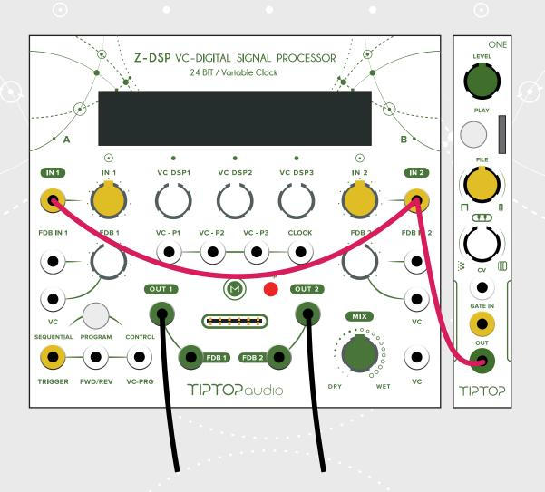
Using a Stackcable plug your sound source into both IN1 and IN2, set LEVEL knob 1&2 to half way, plug OUT1 and OUT2 to a stereo input on your external mixer or computer audio interface. The Z-DSP effects are mostly stereo so it's important to use both outputs.
