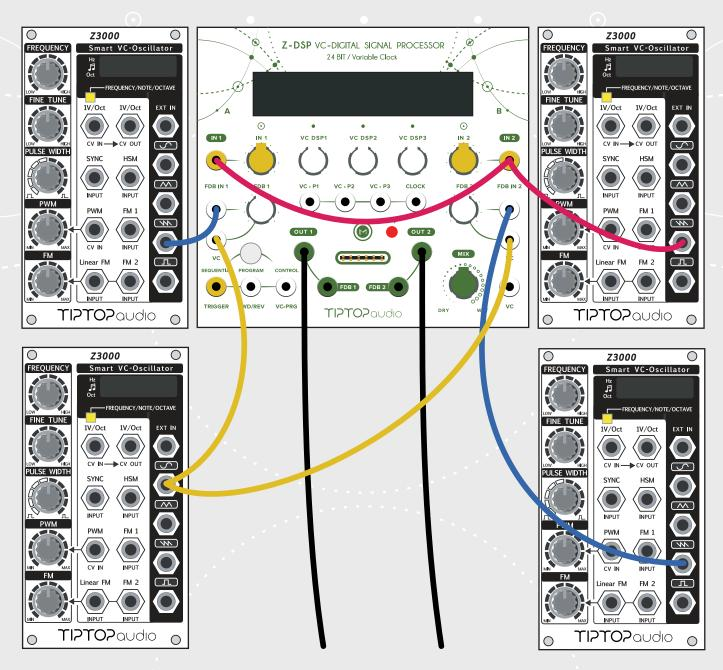
The feedback section has a good amount of gain in it, and will easily cause the module to self-oscillate. This can result in some high frequency 'screeching' which can harm your monitors. So take it easy on that gain knob if you're looking for smoother sounds. Note that the FDB knobs are logarithmic so gain gradually adds up with the turn on the knob, it might be very quiet at the first few steps of the dial, this gives you smoother control of the input gain.
