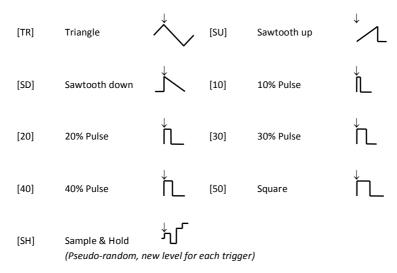
Sets the waveshape of the LFO. All waveshapes modulate CV and/or Aux 1 to any value between 0 to a positive value except triangle, which modulates positive and negative. The downward arrow indicates the default start point, which can be changed with Parameter 53.
