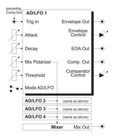
Fig. 1: A-143-1 Controls, Inputs and Outputs
