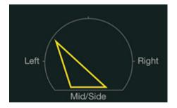
The top point will tilt either direction as the channels become less balanced, and the base will appear narrower to indicate less width.
