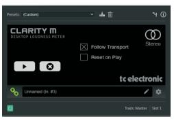
Click the Play/Pause icon to manually start and stop the metering. This button overrules the 'Follow Transport' function. Click RESET to perform a manual reset of the meter.
