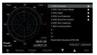
Presets are composed of parameters found on the Edit page. Both RTA and Radar parameters are stored in a preset. Press the 4th button to access the Library menu. Scroll through the available folders with the rotary knob to select the most appropriate category.
