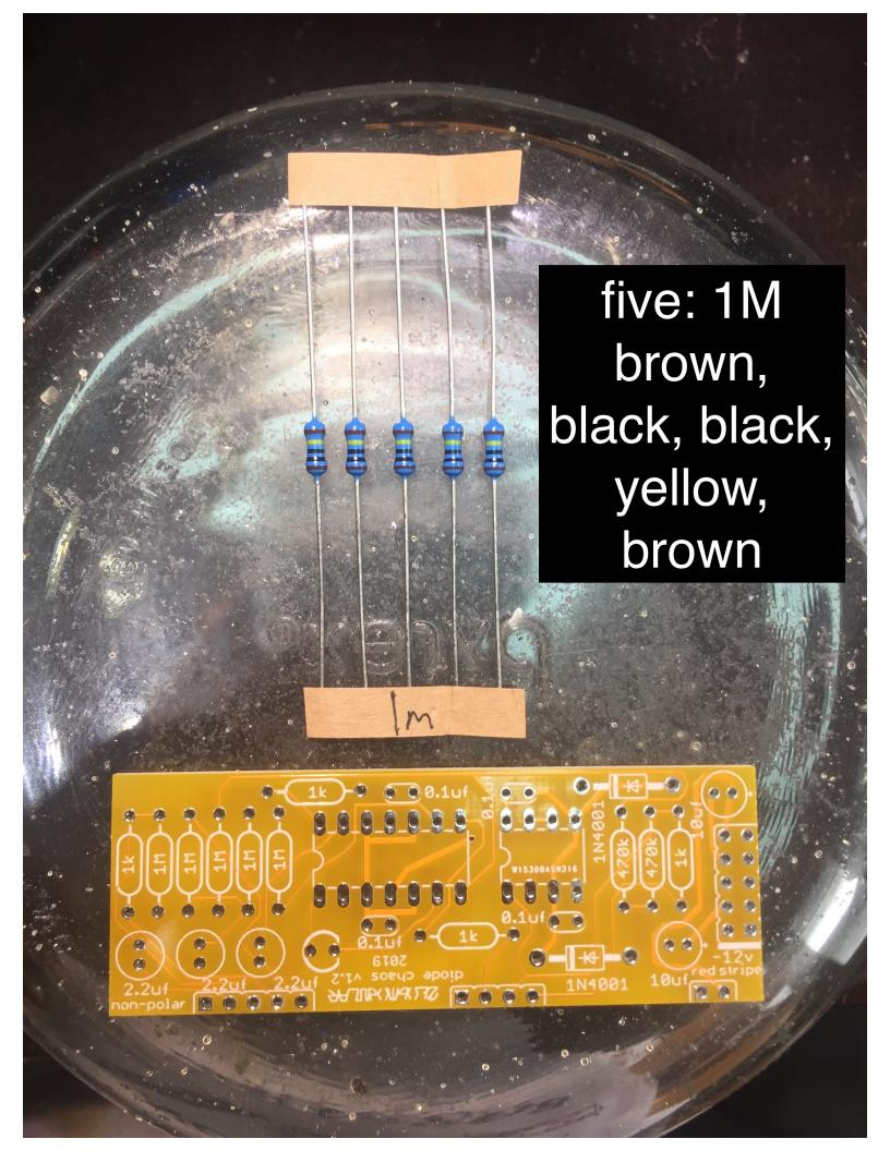
insert the resistors into the side that is silkscreened and bend the legs to hold in place. make sure all resistors are flush with pcb before soldering.
