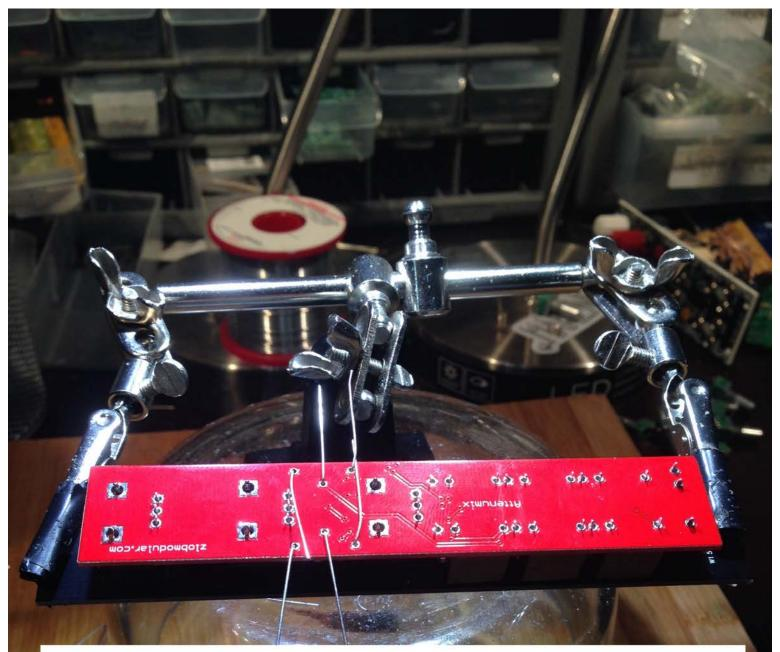
apply tape to helping hands clips to prevent damage to panel. if inserted properly all leads should be poking out to solder. make sure parts are flush
