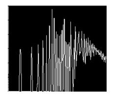
FM amounts at 0, 5, 10 dial positions and their respective spectrums. 100 Hz sawtooth wave is used as a Carried and Modulator.
