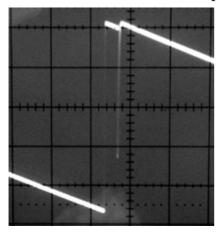
Two teethed saw - to be trimmed CW until the proper saw wave will appear.
