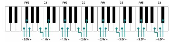
MIDI channel 15 = CV1 calibration MIDI channel 16 = CV2 calibration
