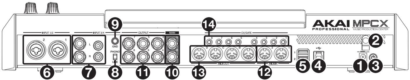
1. **Power Input:** Use the included power adapter to connect MPC X to a power outlet. This must be connected to a power outlet in order for MPC X to power on.
