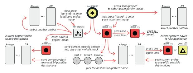
Pressing the PROJECT button will enter the LOAD menu for PATTERNS. Any of the 24 patterns can be selected by pressing the appropriate piano key. Pressing the LAST STEP button being inside that menu will change the load state from PATTERN to PROJECT. Now pressing any of 24 piano keys loads one of the 24 projects.
