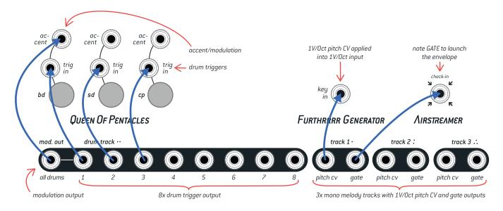
The lowest recognizable MIDI note is C of -2nd octave (MIDI note #0) — its output voltage corresponds to -5V. The highest note is C of 8th octave (MIDI note #120) with the corresponding output voltage of +5V. C3 is the central note that returns exactly 0 volts. It is important to notice that the range of output voltages for any CV output is limited to -5V ... +5V range.
