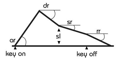
The sound starts when the key is depressed, a process called 'key on'. The sound has an attack, a strong primary decay, followed by a slow secondary decay. The sound continues this secondary decay until the key is released, a process called 'key off'. The sound then begins a rapid final decay, representing for example a piano note after the key has been released and the damper has come down on the strings.
